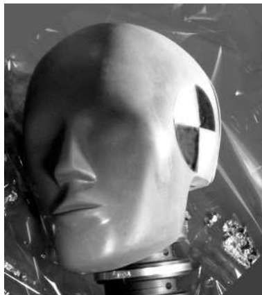
Figure 1.1. Crash test dummies carry artificial landmarks to improve the accuracy of motion measurements from images (Photo courtesy of NASA)
